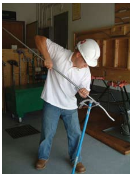
On The Cover: JAC Pre-Apprentice bending 1/2" thin wall conduit
